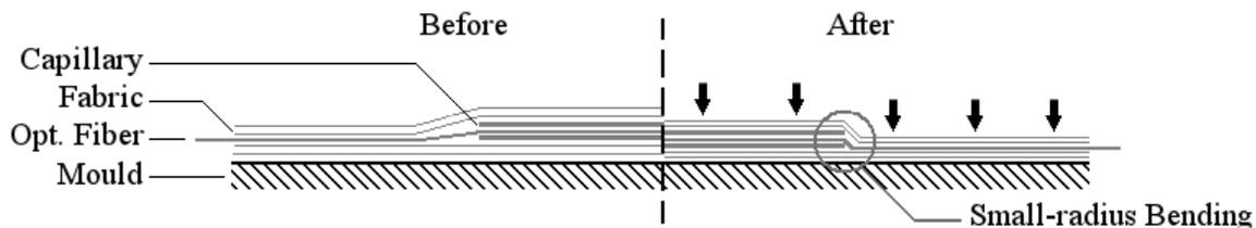
Fig. 4 Bending of the optical fiber by fabric compaction: before and after compaction.
