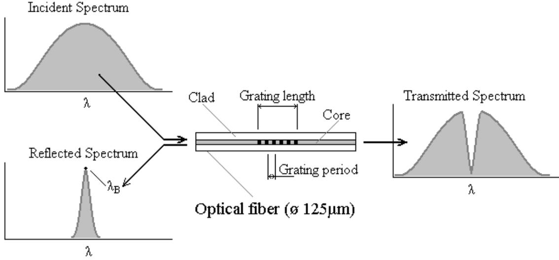
Fig. 1 The fiber Bragg grating structure.
