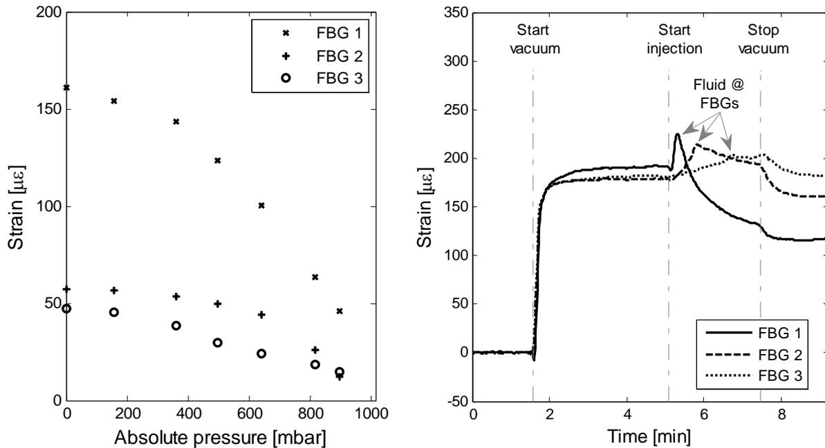
Fig. 3 Initial tests: effect of fabric compaction (left) and flow-front propagation (right).
